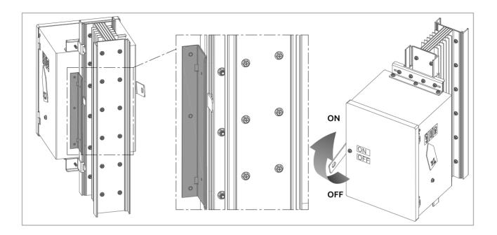
7. Test "ON" and "OFF" to ensure mechanism interlock is in good condition. PIU complete installed.
