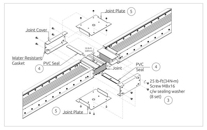
Figure 8.1 Assembly of outdoor busway joint. Correct way to assembly of joint shields is illustrated.
