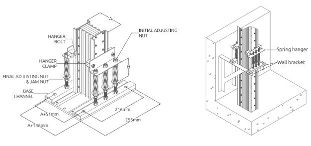
Figure 13.1 Rigid and spring hanger installation
