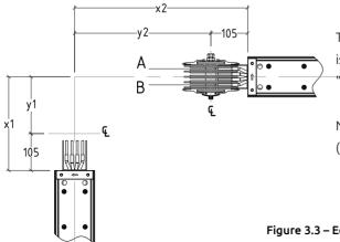
The nominal dimension "y1" and "y2" of the elbow unit is obtained by subtracting 210mm from the dimension "x1" and "x2" measured.
