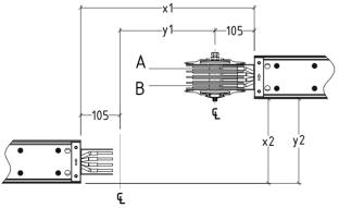
The nominal dimension "y1" of the elbow unit to be ordered is obtained by subtracting 210mm from the dimension "x1" measured. The "x2" is the nominal dimension.
