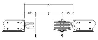
The nominal dimension "y" of the feeder unit is subtracting 210mm from the dimension "x" measured. Example dim. x = 1523 - 210 = 1313mm dim "y".
