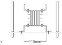
Figure 12.1 Dimension between drop rods for dual-hanger installations.
